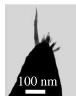
Tip from diamond-like carbon (DLC) grown on the probe apex is shorter and much sharper (tip radius ~1 nm).
