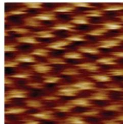
Closed loop (CL) sensors are essential for correct probe repositioning and manipulations. Because CL sensors put some electronic noise they usually are not available below 100 nm. NTEGRA Thermo allows CL correction even below 10 nm. Here is atomic lattice of mica imaged with CL sensors.
